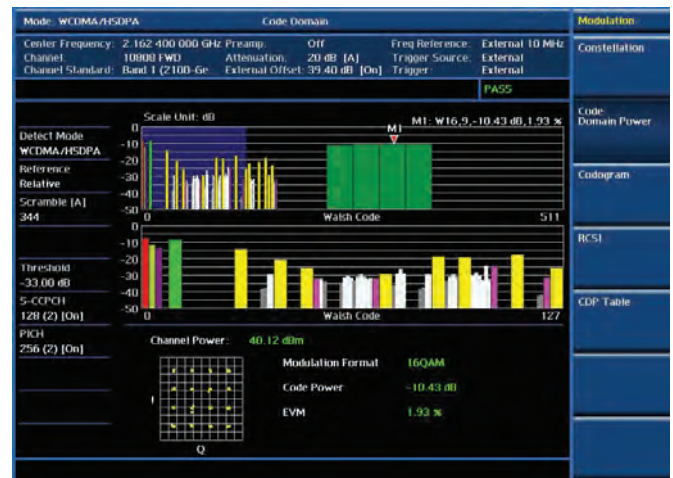
Modulation analysis — Code Domain Power
