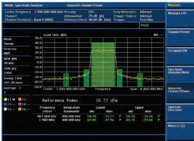
RF test — Adjacent Channel Power
