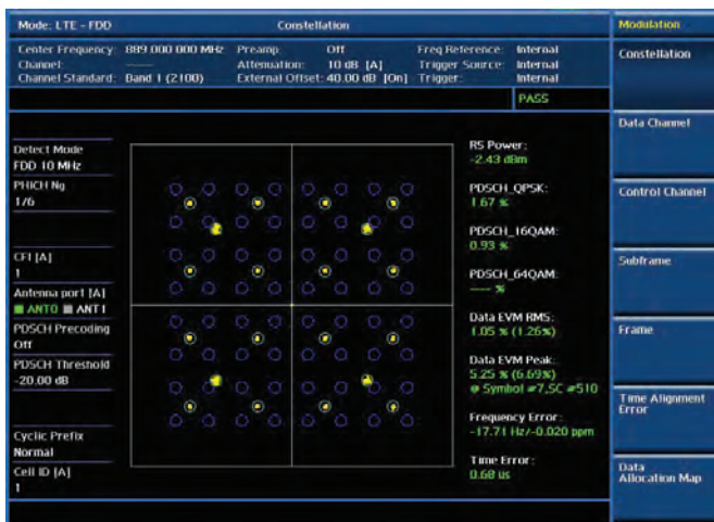
Modulation analysis — Data Constellation
