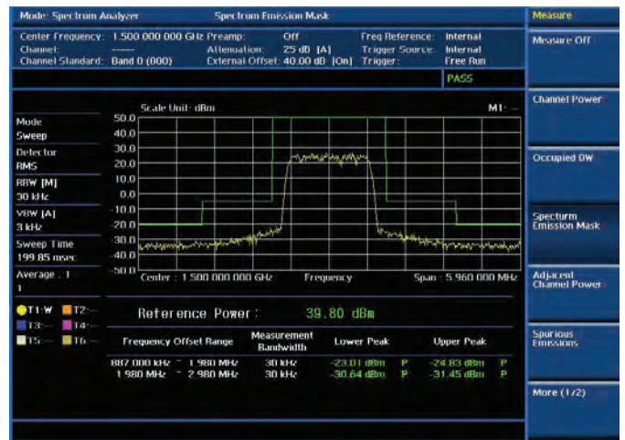
RF test — Spectrum Emission Mask
