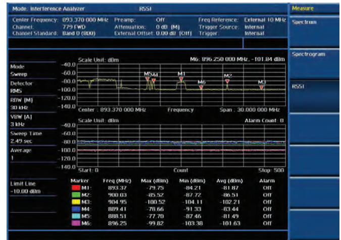
Interference analysis test — RSSI
