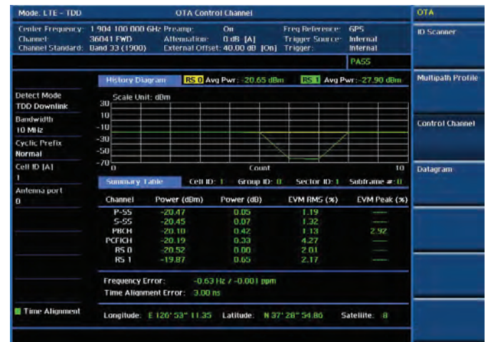
OTA analysis — Control Channels
