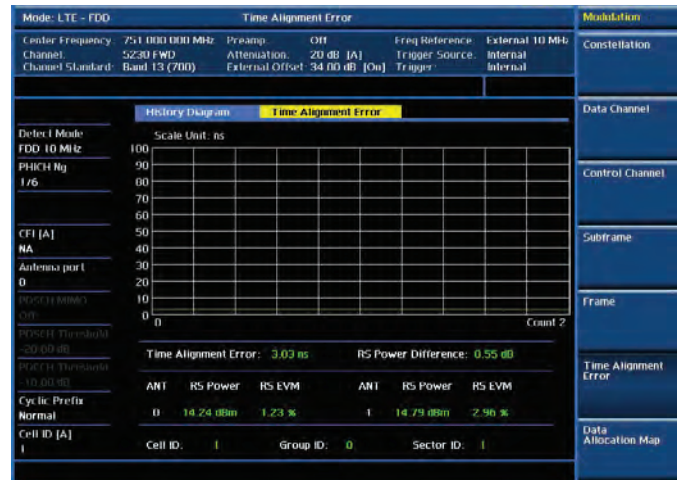
Modulation analysis — Time Alignment Error
