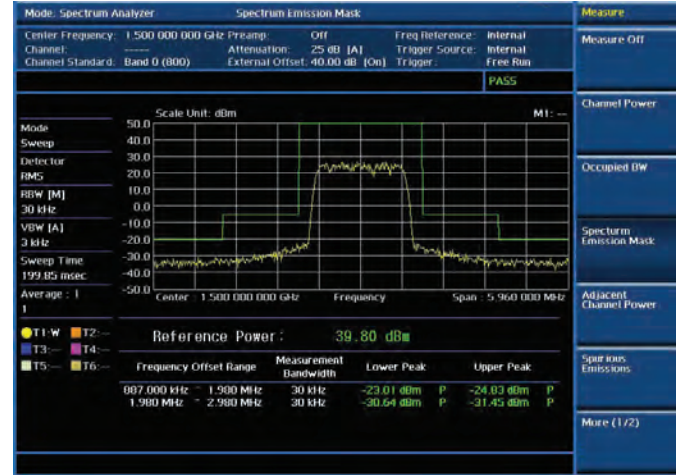
RF analysis — Spectrum Emission Mask
