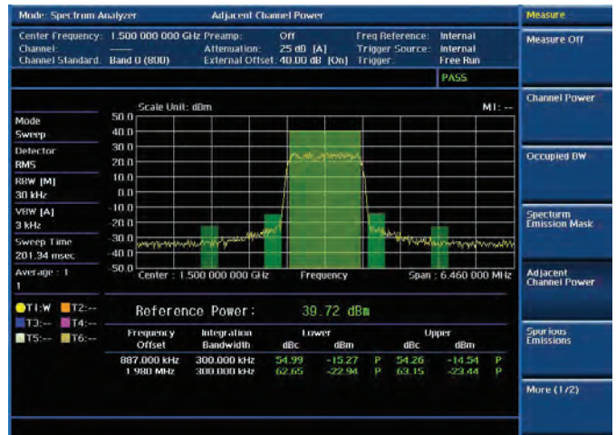
RF analysis — Adjacent Channel Power
