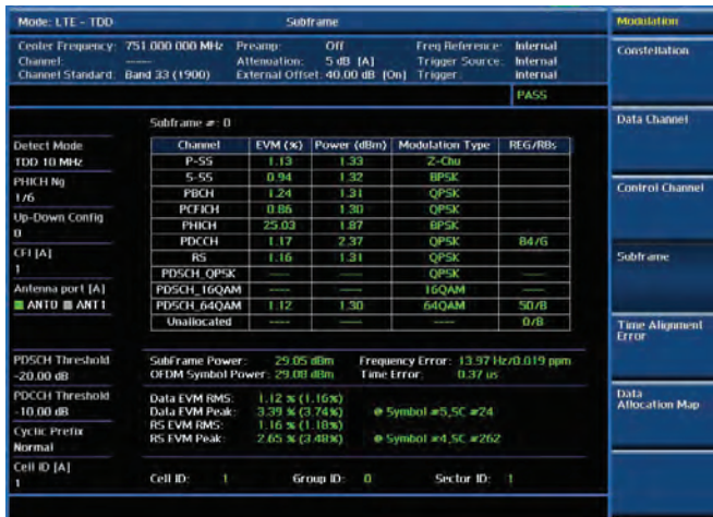
Modulation analysis — Subframe
