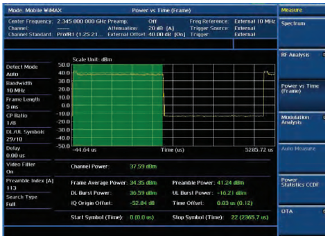
Modulation analysis — Power vs. Time (Frame)
