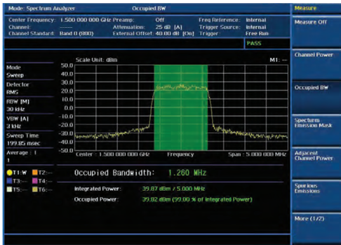
RF analysis — Occupied Bandwidth
