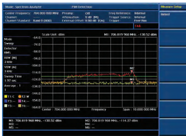
RF test — PIM Detection
