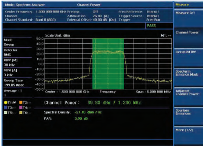
RF analysis — Channel Power
