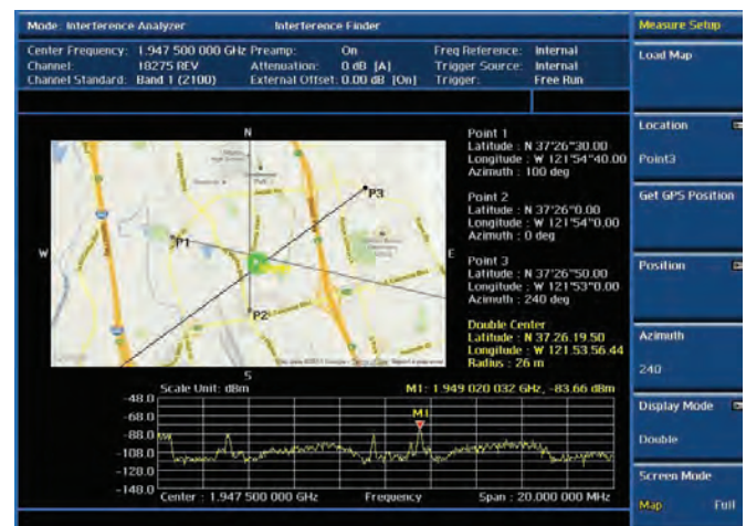
Interference analysis test — Interference Finder
