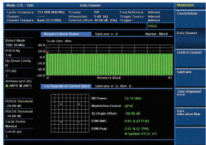
Modulation analysis — Data Channels
