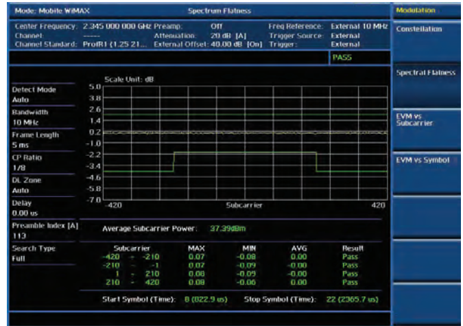
Modulation analysis — Spectral Flatness
