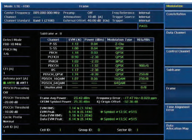
Modulation analysis — Frame
