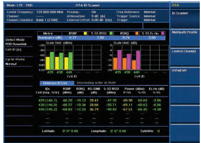
OTA analysis — ID (Channel Scanner)
